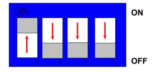
Figure 3.5: DIP switch setting
